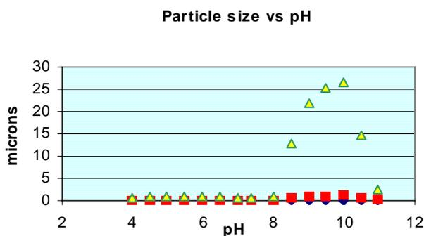
In this unstable region the measured size depends on factors such as the pump speed or stirring rate, since the shear forces from the flow limit the floc size. The size will also depend on factors such as the particle concentration and the time between measurements.
